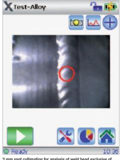
3 mm spot collimation for analysis of weld bead exclusive of ioined material
